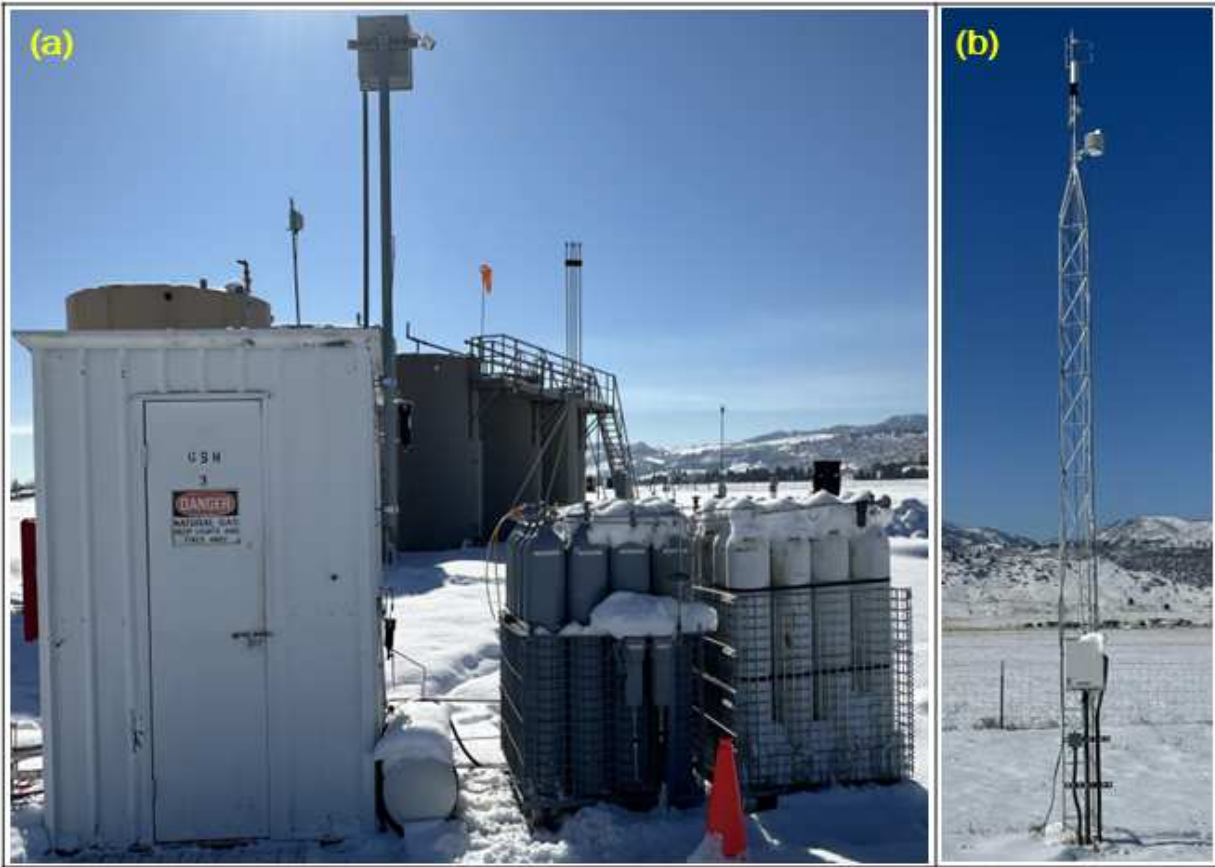
Figure 2.8: (a) The gas supply house (GSH) that regulates the controlled release of gas to emission points embedded within equipment units in well pads 4 and 5. The figure also shows the gas storage bottles provided to augment the onsite gas storage capacity for releases to the well pads. (b) The \approx 7\text{m} weather station located near the western end of the test center.
