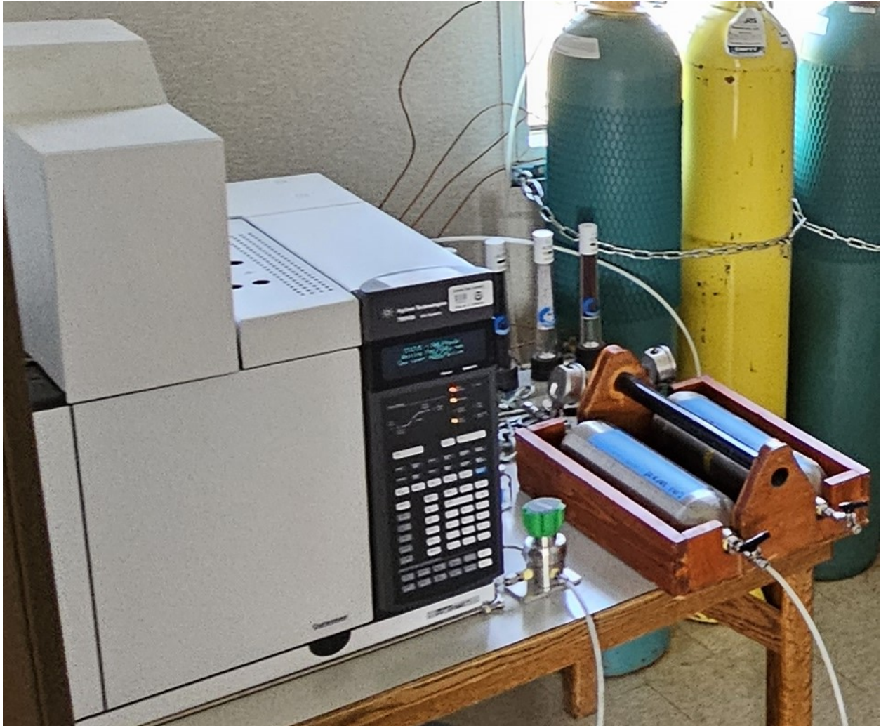
Figure A.1: Shows the gas chromatography device used to identify and analyze the species and chemicals that make up the gas supply at METEC. The figure also shows the canisters used to collect gas samples from the onsite gas storage cylinders for species composition analysis.
