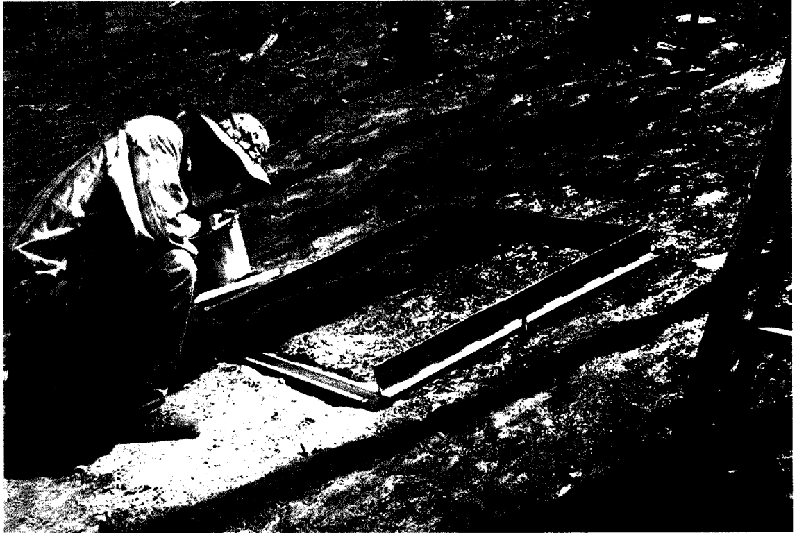
Figure 3. Picture of the frame used to isolate each 1 m 2 plot and the trough used to collect runoff.
