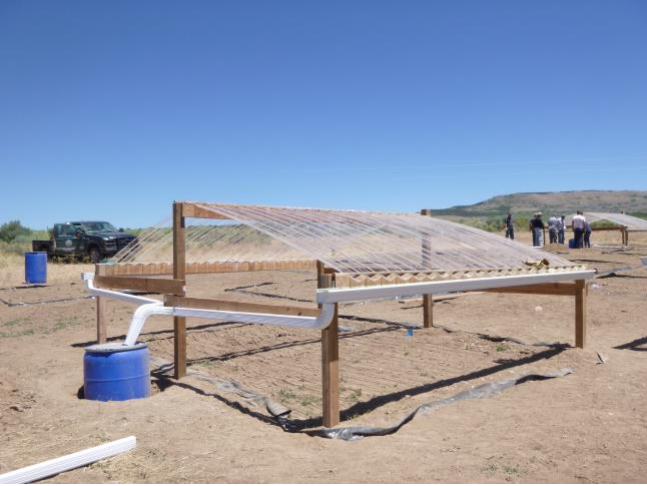
Figure A.1.1: Rainfall exclusion shelter used to impose drought treatments on plots.
