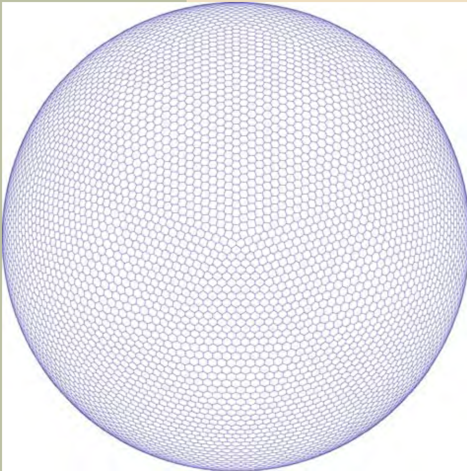
Figure 1: The icosahedral grid mesh composed of 10242 Voronoi cells (at grid refinement level 5).
