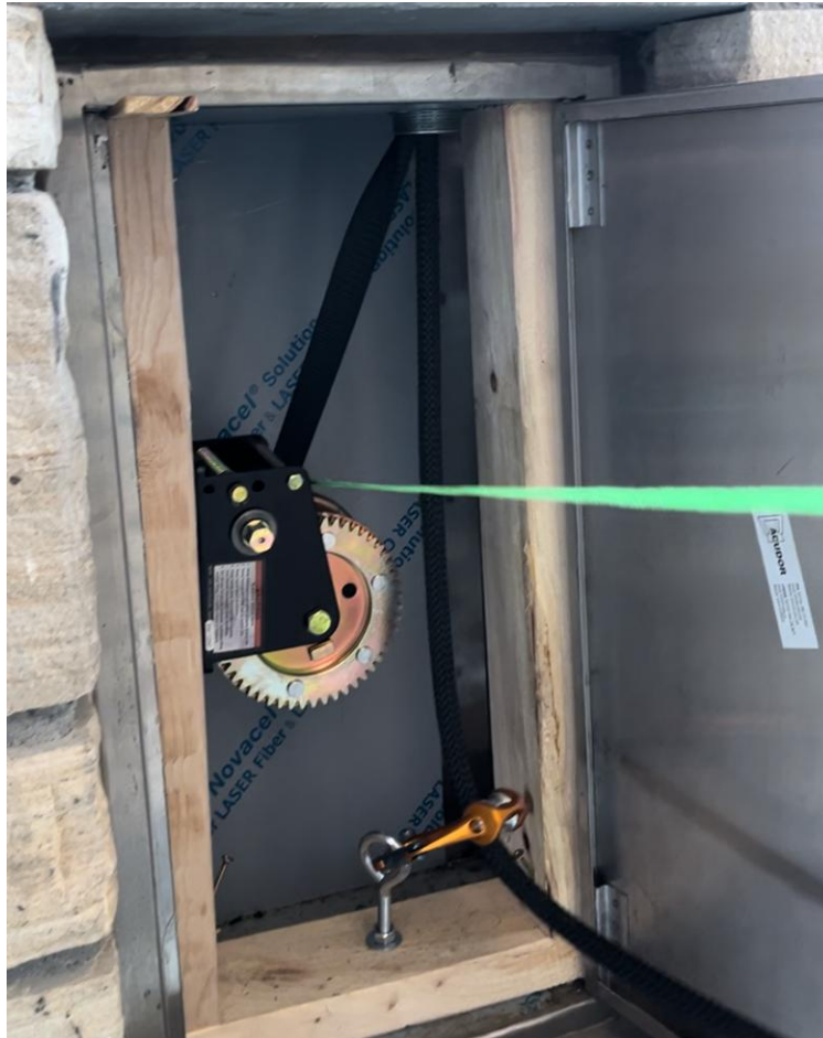
Figure 2: Ratchet System Proof of Concept
