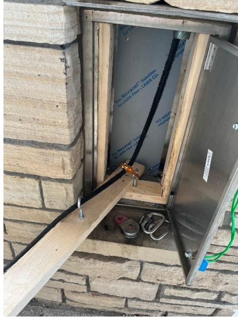
Figure 6: Prototype of rope redirection wooden frame
