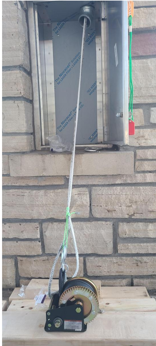
Figure 5: Ratchet prototype mounted outside of box
