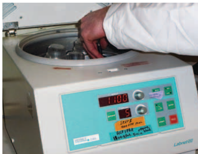
Centrifuge used to spin the blood as part of the process leading to the harvest of PRP.
