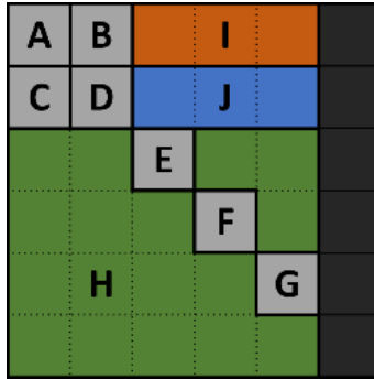
Fig. 6.4. Basis function weight grids. Function weights in A-G were given to network as input. Weights in regions H, I, and J were predicted by the network.
