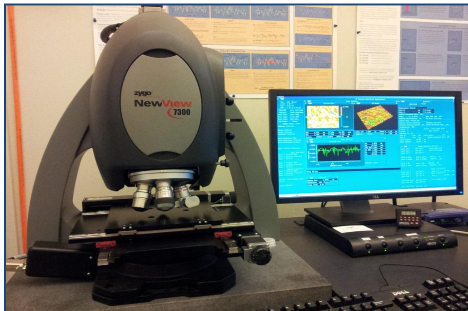
Figure 2.1: The Zygo New View Scanning White Light Interferometer used for data acquisition and processing.
