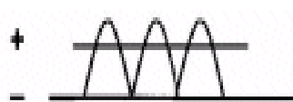
Fig. 3 Diode Bridge converts AC to DC and the Bus then smoothes signal
