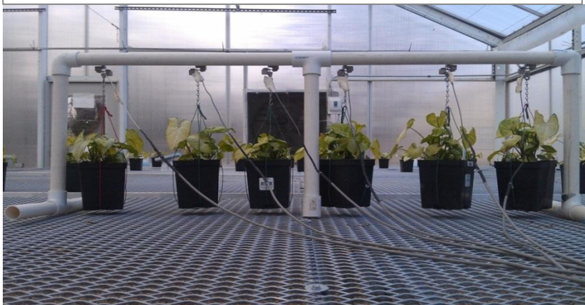
Fig. 14 Hanging lysimeter setup used to determine water loss rate characteristics in both VFD and On/Off fan greenhouses simultaneously.
