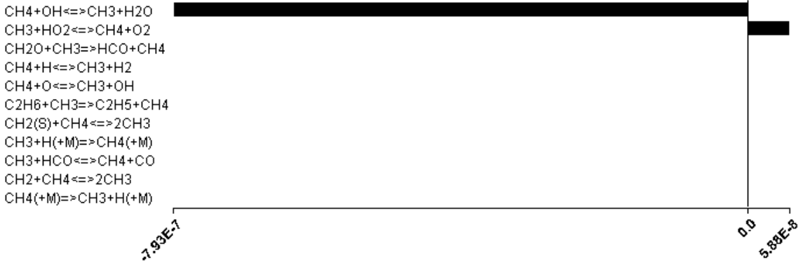
Figure 22. Rates of production of all reactions that influence the CH 4 equilibrium at the selected solution point for MD19. Figure obtained from CHEMKIN.
