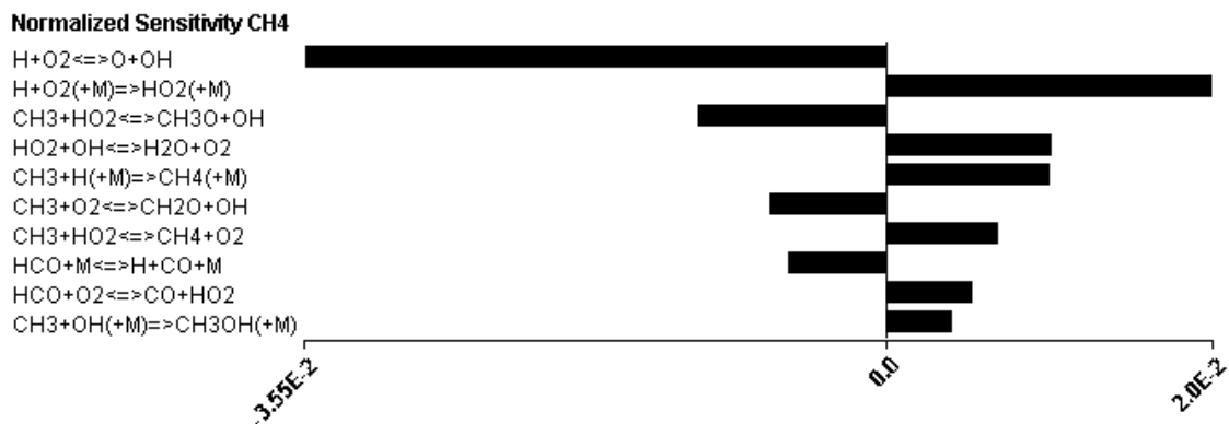
Figure 17. Sensitivity of selected species in relation to the rates of reactions of the mechanism for Zsely 50s 251rxn. Figure obtained from CHEMKIN.
