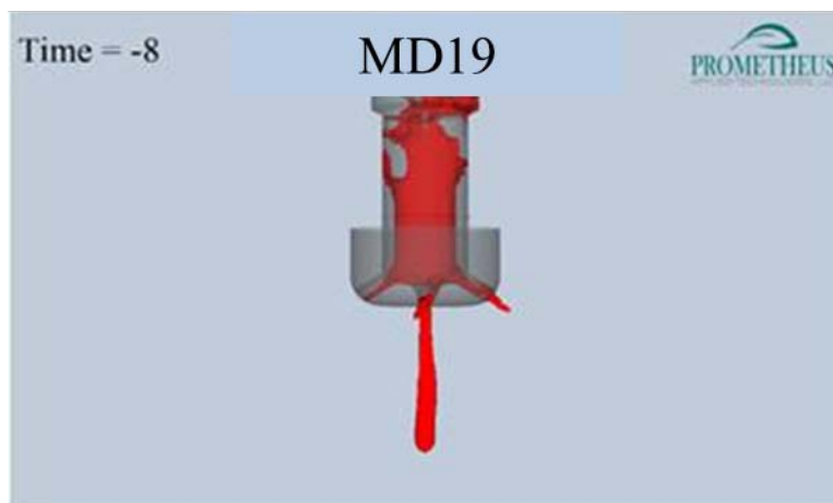
Figure 42. Development of flame torches at 16 CAD after spark MD19.
