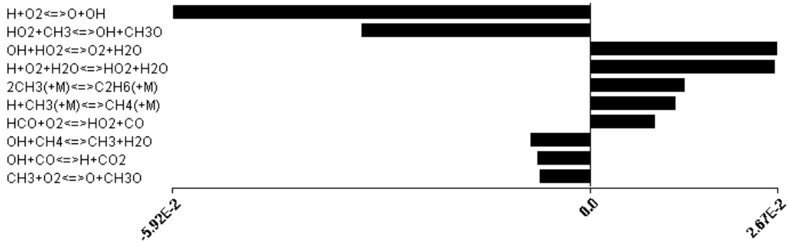
Figure 20. Sensitivity of selected species in relation to the rates of reactions of the mechanism for DRM22. Figure obtained from CHEMKIN.
