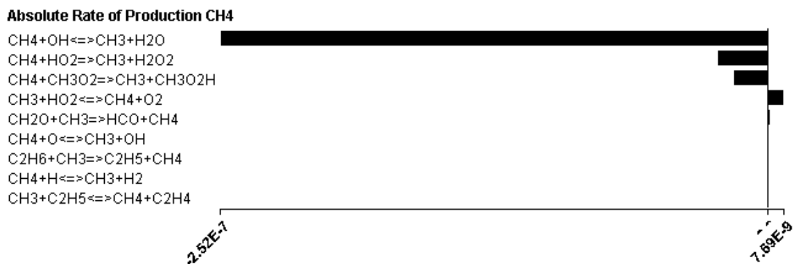
Figure 25. Rates of production of all reactions that influence the CH 4 equilibrium at the selected solution point for Nagy21. Figure obtained from CHEMKIN.
