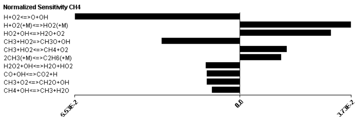
Figure 26. Sensitivity of selected species in relation to the rates of reactions of the mechanism for Nagy21. Figure obtained from CHEMKIN.
