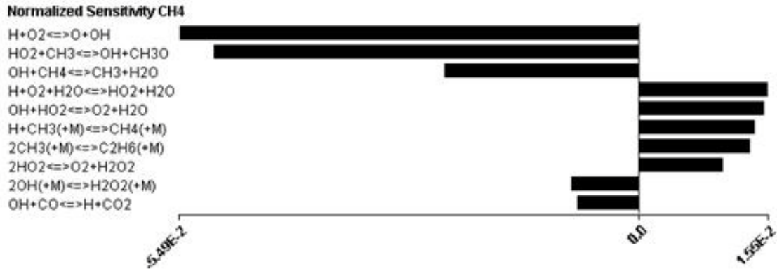
Figure 14. Sensitivity of selected species in relation to the rates of reactions of the mechanism for GRI-Mech3.0. Figure obtained from CHEMKIN.
