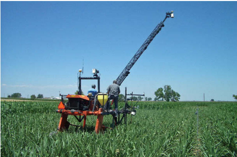
Figure 3. High Boy reflectance tractor measuring corn canopy reflectance and temperature to determine the level of stress and water use.
