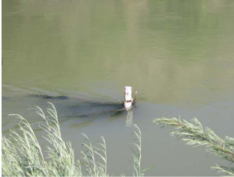
Figure 2. Weeds can be an issue at the Elephant Butte stream gaging site
