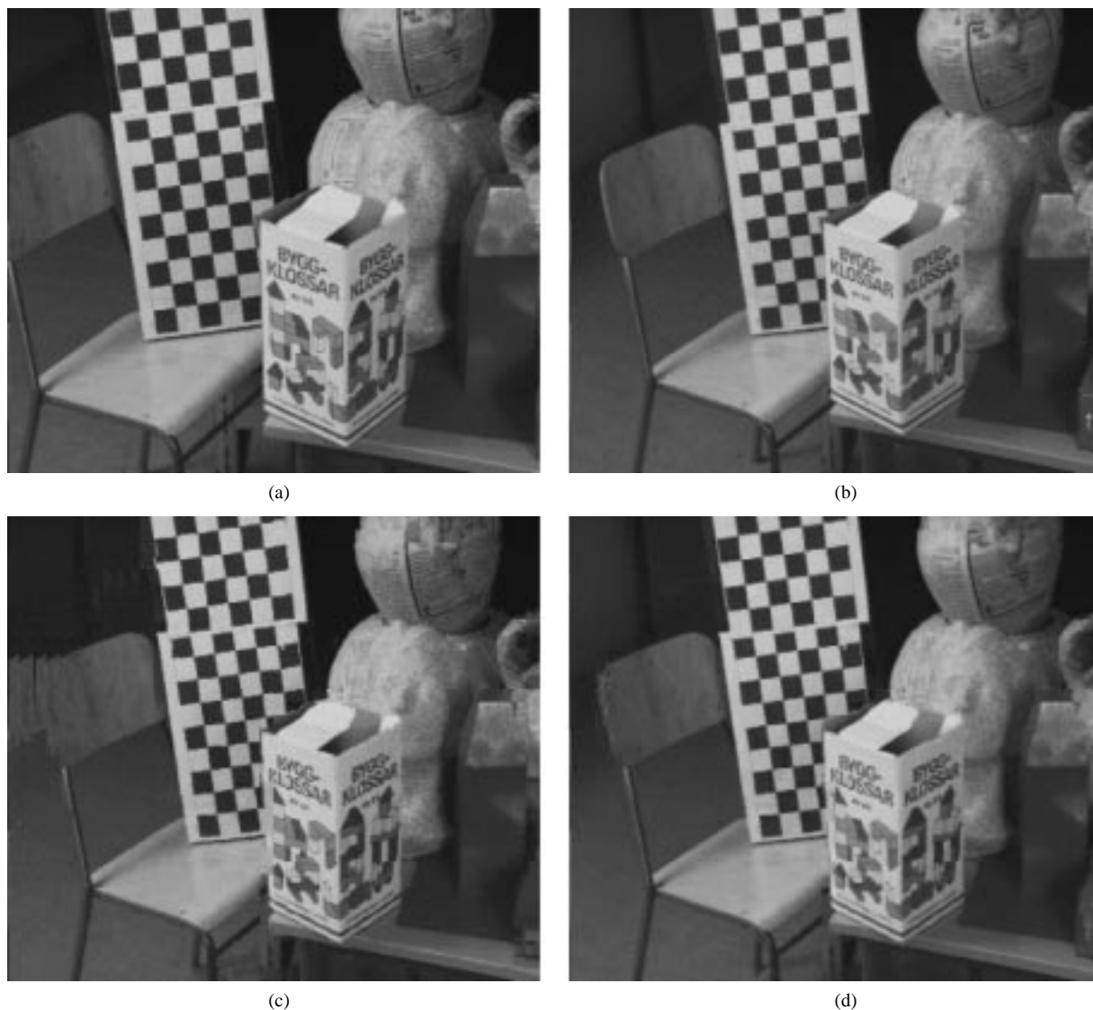
Fig. 2. (a) and (b) Original stereo image pair of "Chair." (c) Reconstructed image using the standard block-matching. (d) Full-order (four weights) filtering.
