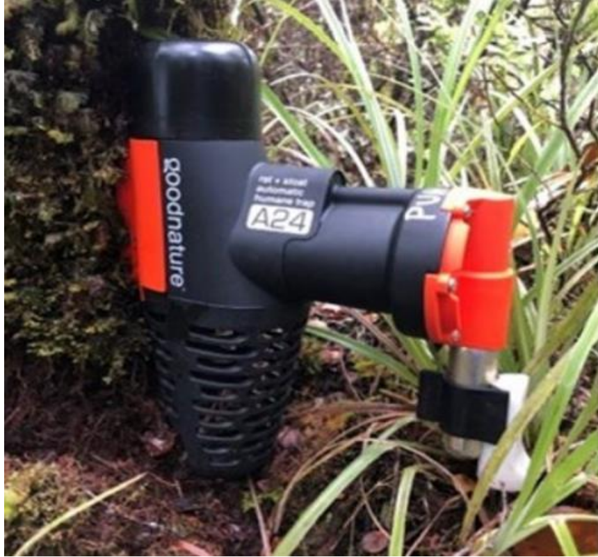
Figure 1.2. Goodnature A24 rat trap with plastic blocker attached. These traps were used to control rats in the treatment plots. Each plastic blocker was secured via zip ties to the opening of the trap to prevent non-target kills. Photo property of KFBRP.
