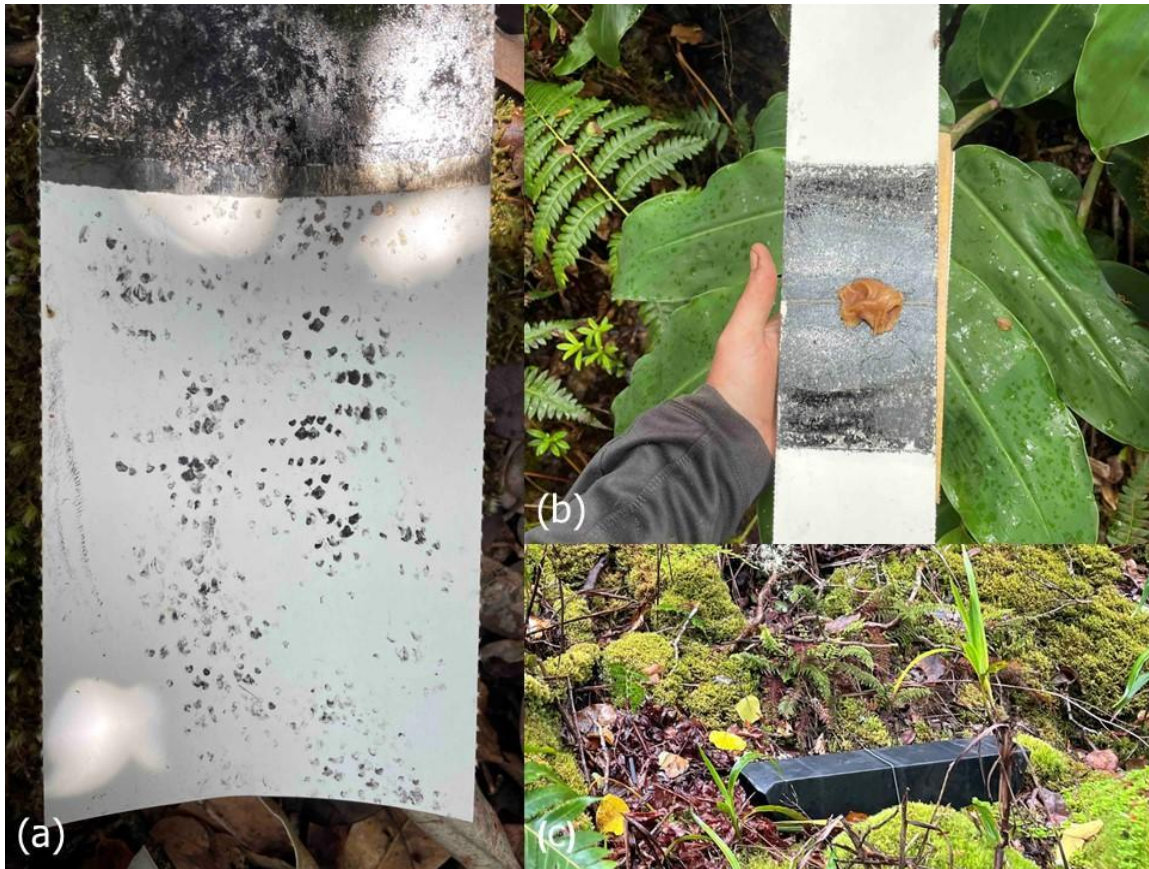
Figure 1.3. Tracking tunnels were used to measure relative rat abundance in control and treatment plots. Relative abundance was measured by tracking the presence or absence of rat footprints using a track pad (a), which was baited with peanut butter (b) and placed on the forest floor (c). Photos property of KFBRP.
