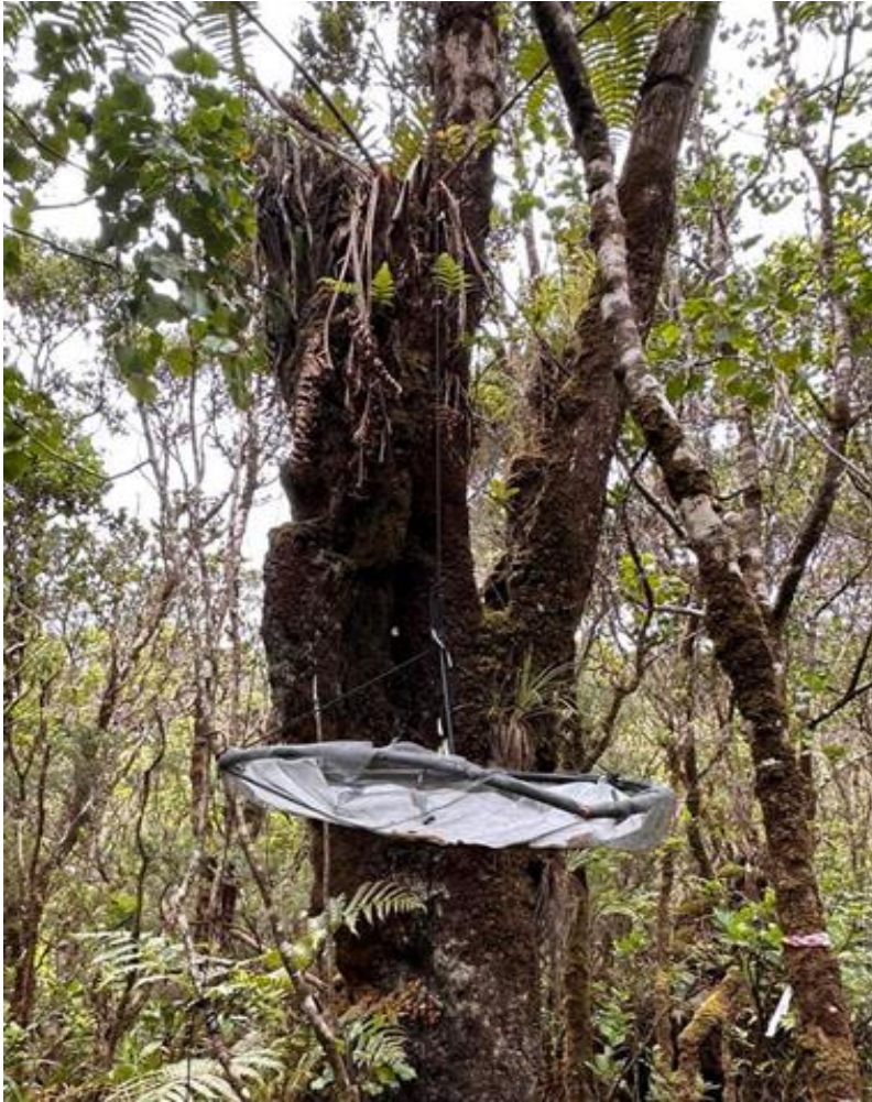
Figure 2.3. Example of a seed rain trap that was used to assess seed rain in the presence and absence of rodent control in Kaua‘i, Hawai‘i. Seed traps consisted of 1m diameter mesh baskets with a silkscreen. Traps were hung from trees in the understory to collect seed rain in the forest.
