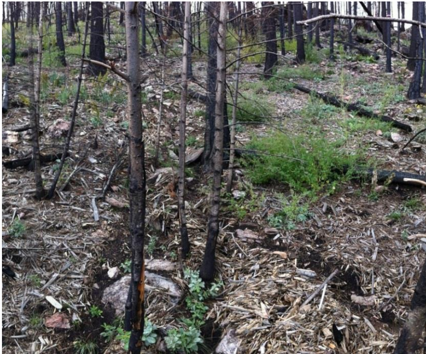
Figure 3.10: Rills approximately 10-20 cm deep through wood mulch after the 09/2013 event. Photo is facing uphill from the sediment fence at swale HU1.
