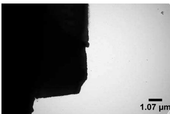
Figure 2.25. Representative micrograph of 2FGS crystal loaded with 10 nm AuNPs. These crystals tend to be too thick for electron microscopy.
