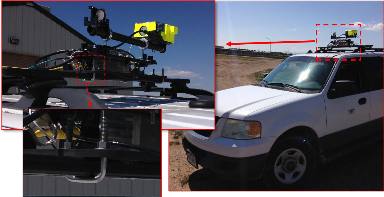
Figure 5.3: Installation of the ammonia sensor on an SUV.
