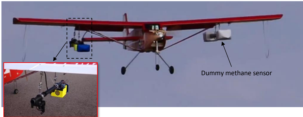
Figure 5.10: The real ammonia and dummy methane sensors on the UAS during a flight.
