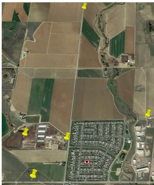
5.7: A map of the dairy facility and surrounding lands. The pins show the 5 individual measurements locations. Site 1 is co-located with the anemometer and is the closest site to the pens. The other spots were selected based on the wind direction measured by the anemometer.
