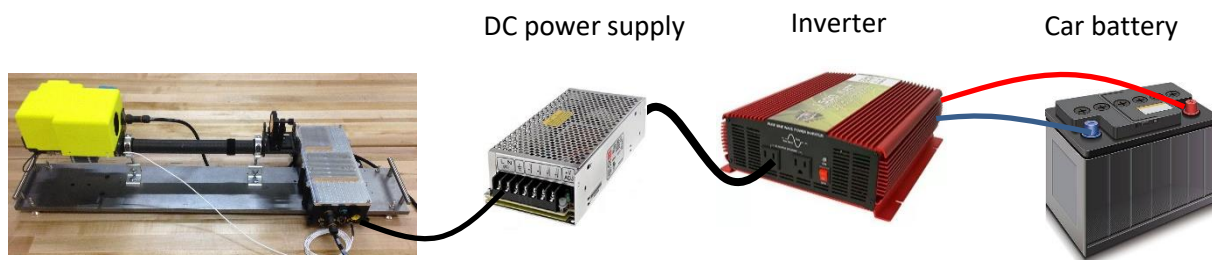
Figure 5.1: The sensor is powered using the car battery, a power inverter, and a DC power supply.
