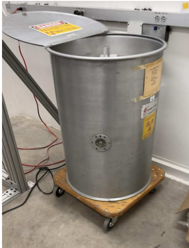
Figure 2.6 Neutron Howitzer - PuBe Housing
