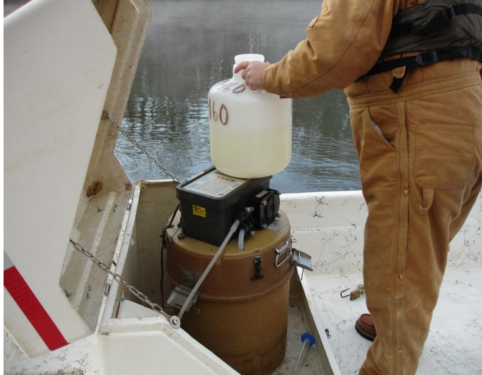
Figure 2. The weekly 10 L composite sample collection and ISCO sampler calibration at River Mile 160 (RM-160)
