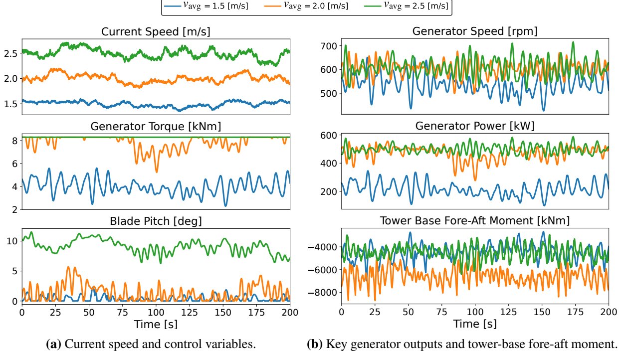
Figure 3.3: Time series plot of key signals in the below-rated (1.5 m/s), transition (2.0 m/s), and above-rated (2.5 m/s) regions obtained using \mathbf{x}_{c,init} .
