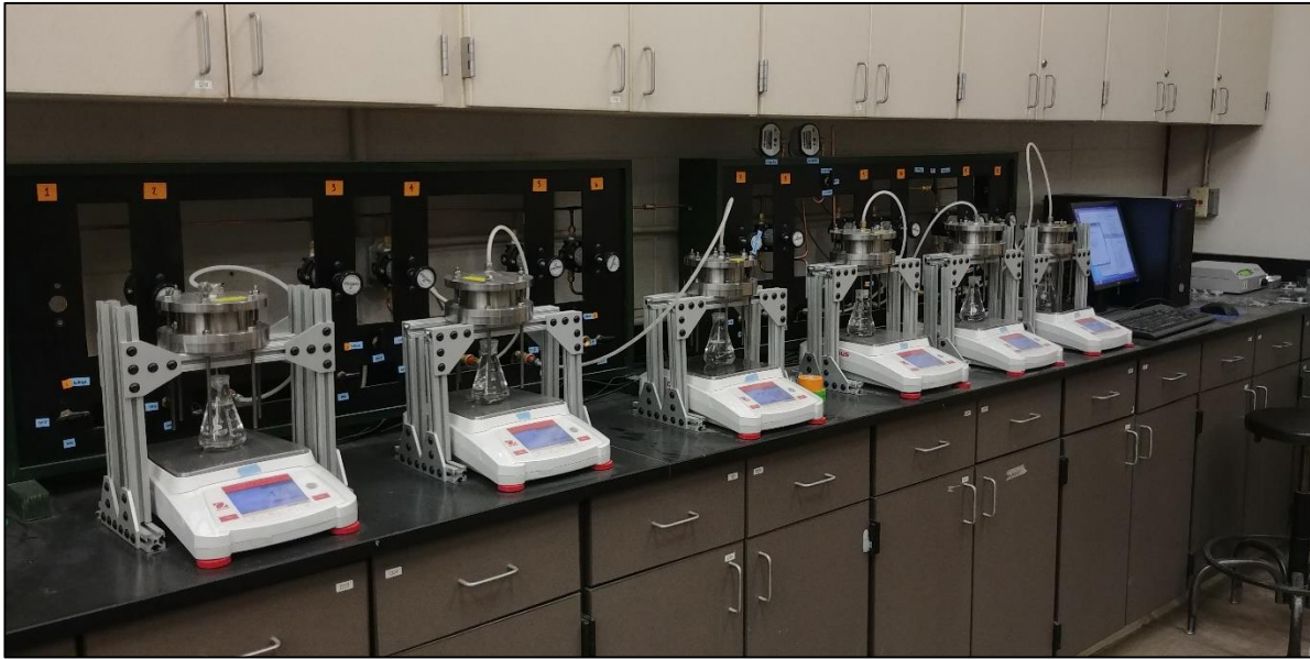
Figure 1.5 - Running pressure plate tests.
