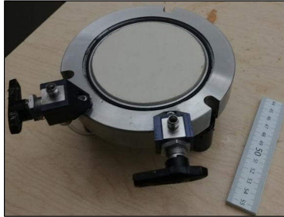
Figure 2.3 - The bottom plate of the compression apparatus containing a high air entry (HAE) ceramic disk.
