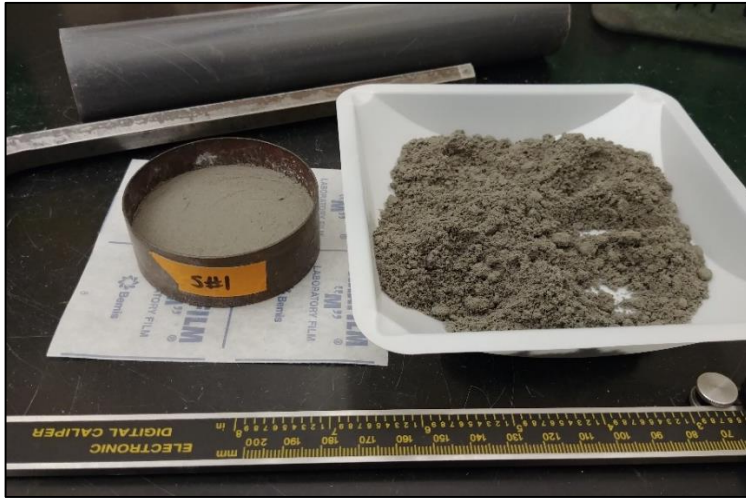
Figure 1.3 - A pressure plate specimen compacted inside a ring.
