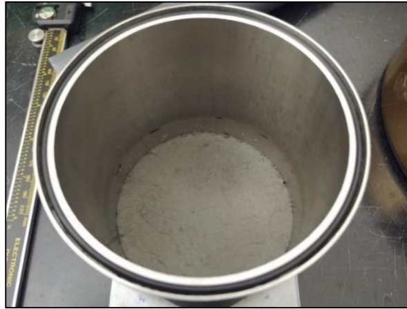
Figure 2.4 - A filter cake specimen getting compacted to the marked line of 25 mm inside the compression apparatus cell.
