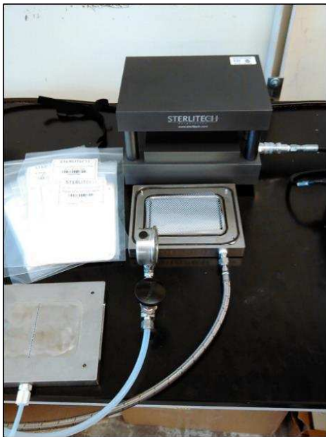
Figure 4.20: Large Scale Reverse Osmosis - SEPA Cell
