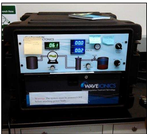
Figure 4.1: EC Control Unit
