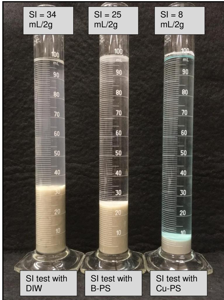
**Fig. 5.14.** Photograph of swell index tests conducted with non-hydrated bentonite (i.e., exhumed dry from as-received GCL) in de-ionized water (DIW), B-PS, and Cu-PS.
