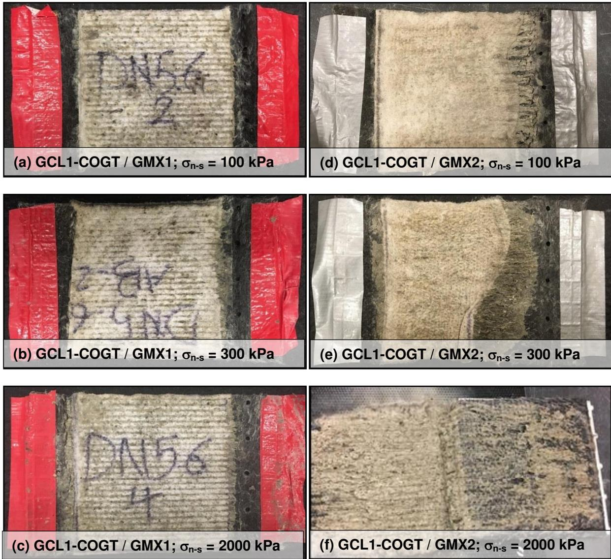
**Fig. 3.14.** Post shear pictures of GCL1 specimen in DC-IF tests on (a) GCL1-COGT/GMX1 at  $\sigma_{n-s} = 100$  kPa, (b) GCL1-COGT/GMX1 at  $\sigma_{n-s} = 300$  kPa, (c) GCL1-COGT/GMX1 at  $\sigma_{n-s} = 2000$  kPa, (d) GCL1-COGT/GMX2 at  $\sigma_{n-s} = 100$  kPa, (e) GCL1-COGT/GMX2 at  $\sigma_{n-s} = 300$  kPa, and (f) GCL1-COGT/GMX2 at  $\sigma_{n-s} = 2000$  kPa
