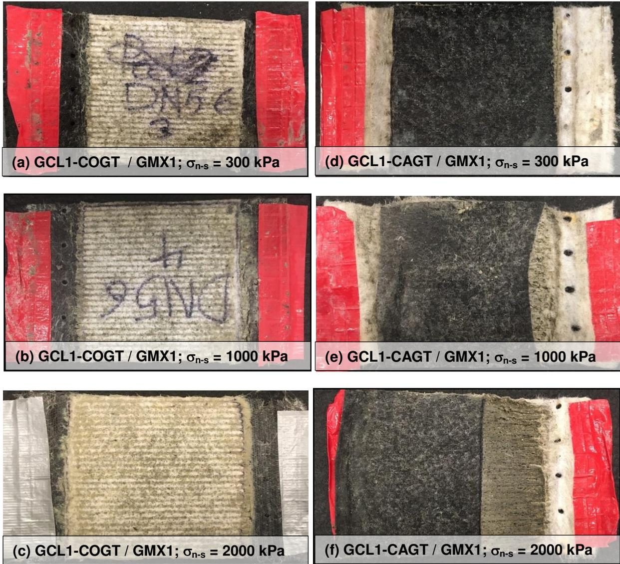
**Fig. 3.10.** Post shear pictures of GCL1 specimen in DC-IF tests on (a) GCL1-COGT/GMX1 at  $\sigma_{n-s} = 300$  kPa, (b) GCL1-COGT/GMX1 at  $\sigma_{n-s} = 1000$  kPa, (c) GCL1-COGT/GMX1 at  $\sigma_{n-s} = 2000$  kPa, (d) GCL1-CAGT/GMX1 at  $\sigma_{n-s} = 300$  kPa, (e) GCL1-CAGT/GMX1 at  $\sigma_{n-s} = 1000$  kPa, and (f) GCL1-CAGT/GMX1 at  $\sigma_{n-s} = 2000$  kPa.
