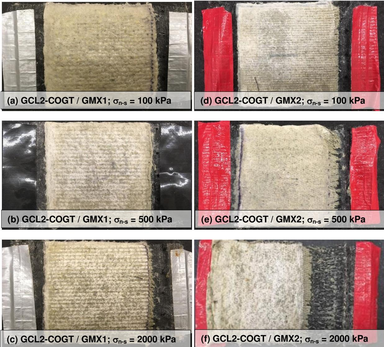
**Fig. 3.16.** Post shear pictures of (a) GCL2-COGT/GMX1 at  $\sigma_{n-s} = 100$  kPa, (b) GCL2-COGT/GMX1 at  $\sigma_{n-s} = 500$  kPa, (c) GCL2-COGT/GMX1 at  $\sigma_{n-s} = 2000$  kPa, (d) GCL2-COGT/GMX2 at  $\sigma_{n-s} = 100$  kPa, (e) GCL2-COGT/GMX2 at  $\sigma_{n-s} = 500$  kPa, and (f) GCL2-COGT/GMX2 at  $\sigma_{n-s} = 2000$  kPa.
