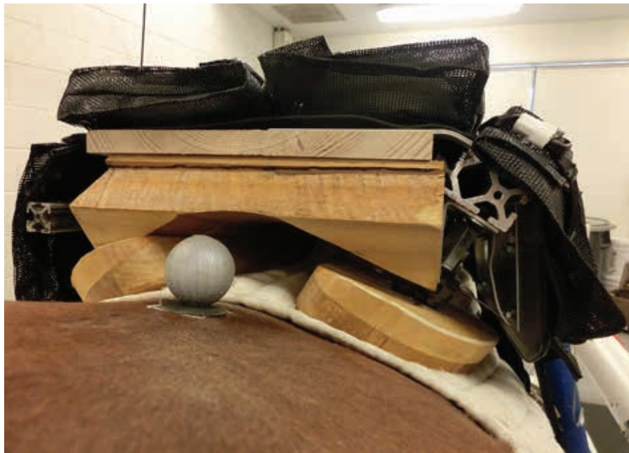
Fig. 1 (above): The instrumented saddle showing induced pressure on the right caudal portion of the saddle. The gap on the right side between the tree (dorsally) and the moveable saddle section (ventrally) represents how the different portions of the saddle are used to induce increased local saddle pressures.
